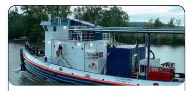
Amogy succesfully <u>launched</u> the first carbon-free, ammonia powered maritime vessel, a tugboat <u>named</u> NH<sub>3</sub> Kraken. Amogy's ammonia cracking technology <u>converts</u> liquid ammonia (NH<sub>3</sub>) into its base elements of hydrogen and nitrogen, and then funnels the hydrogen into a fuel cell. The system is designed for vessels as small as a tugboat and as large as a containership and could also work in other heavy industries.
